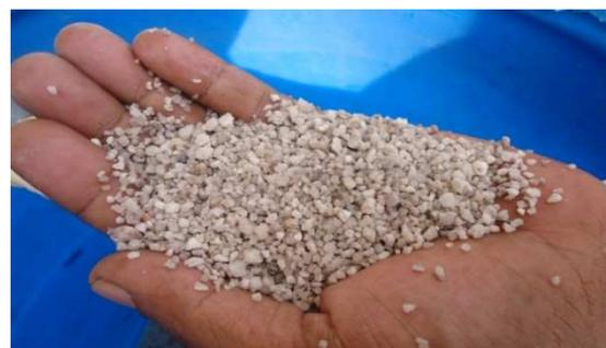
Gambar 3. Photo pasir silica diameter 1,95 mm
